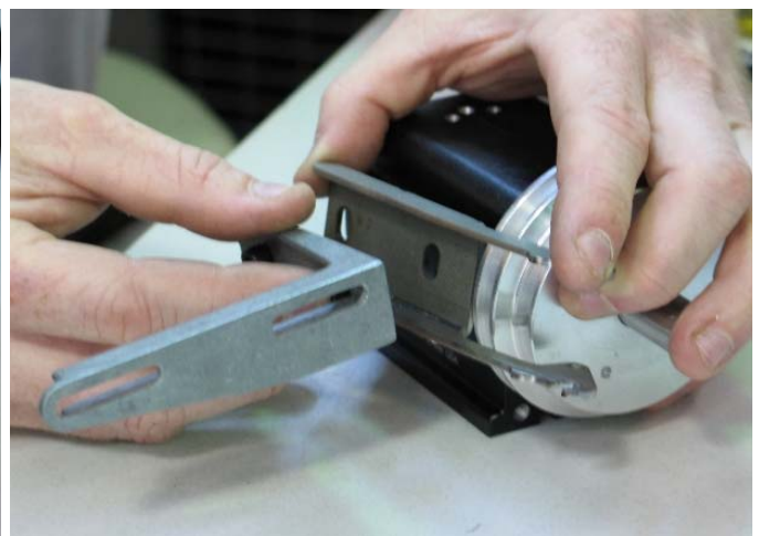
Install Main Bracket & Sherline Motor Mount
