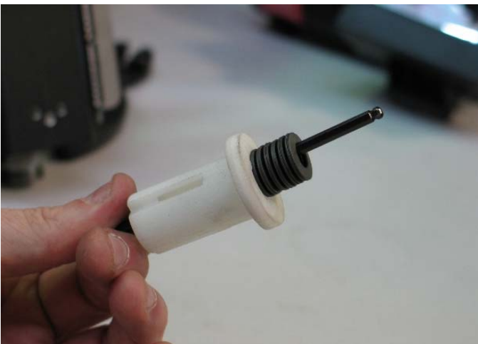
Slide Belleville Springs into Spring Cup
