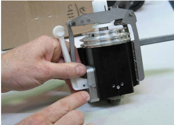
Pin Lever to Lever Mount
