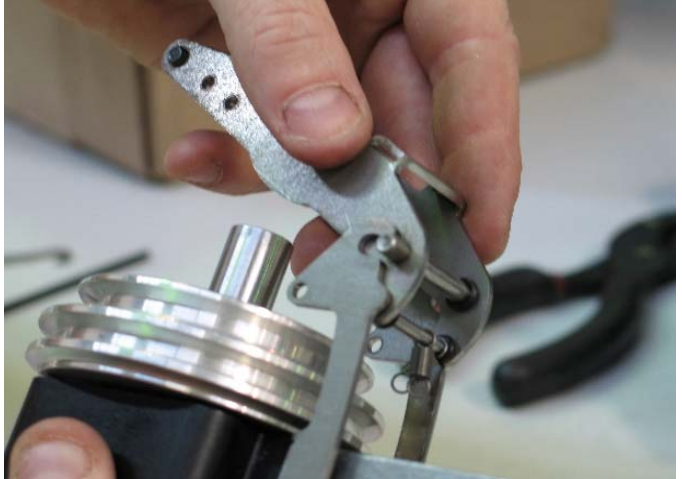
Install Actuator Lever Assembly
