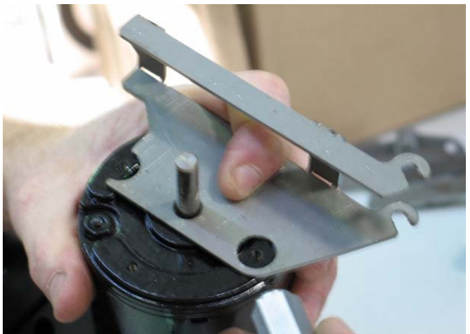
Install Motor Bracket
