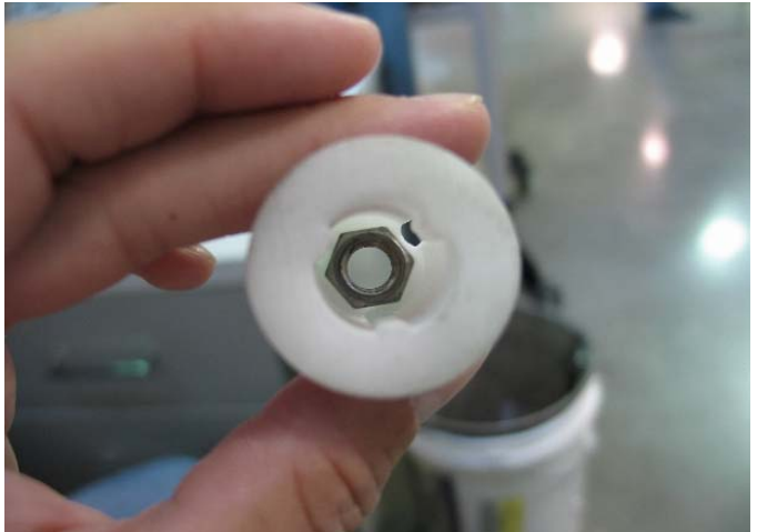
Insert Nut inside Spring Cup
