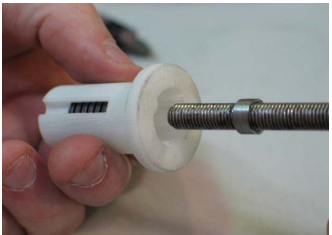
Thread on bushing and install drawbar
