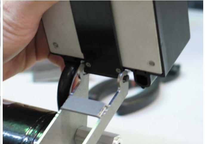
Attach motor control box
