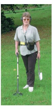
(Tip: The coil is not interchangeable with any other Fisher, so don't try and use coils from other Fisher detectors even if they have the same male plug).
